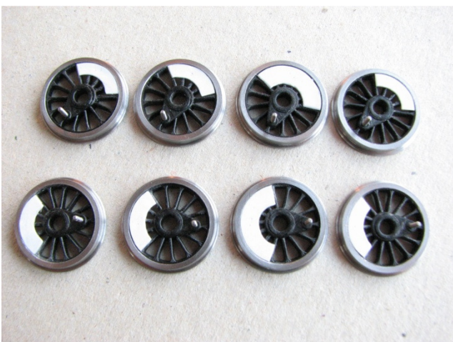
Gibson wheels fitted with crankpins and balance weights.
