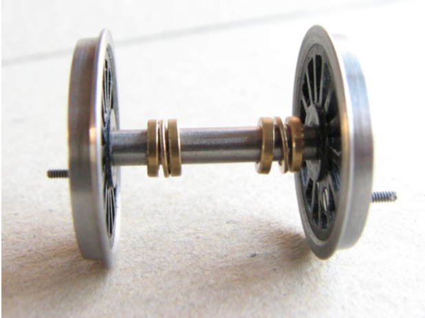
Wheels assembled (first, third and fourth axles).
