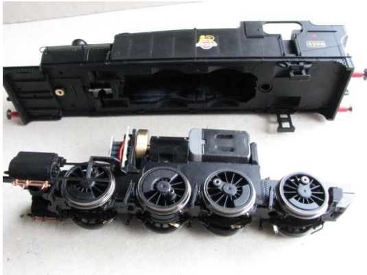
Footplate sprang back and clipped in place with no damage.
