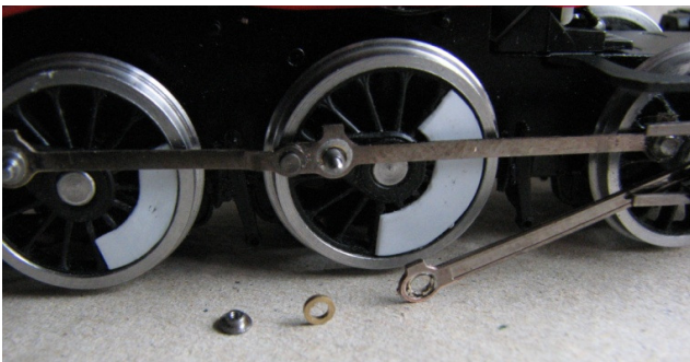
Brass washer to fit between coupling and connecting rod.
