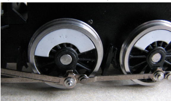
Completed rod assembly.
