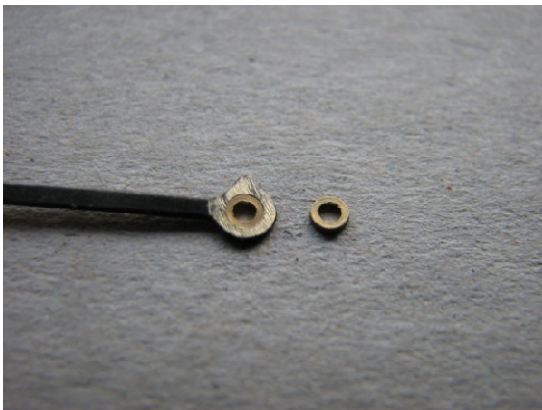
Bush in rod ready for soldering.
